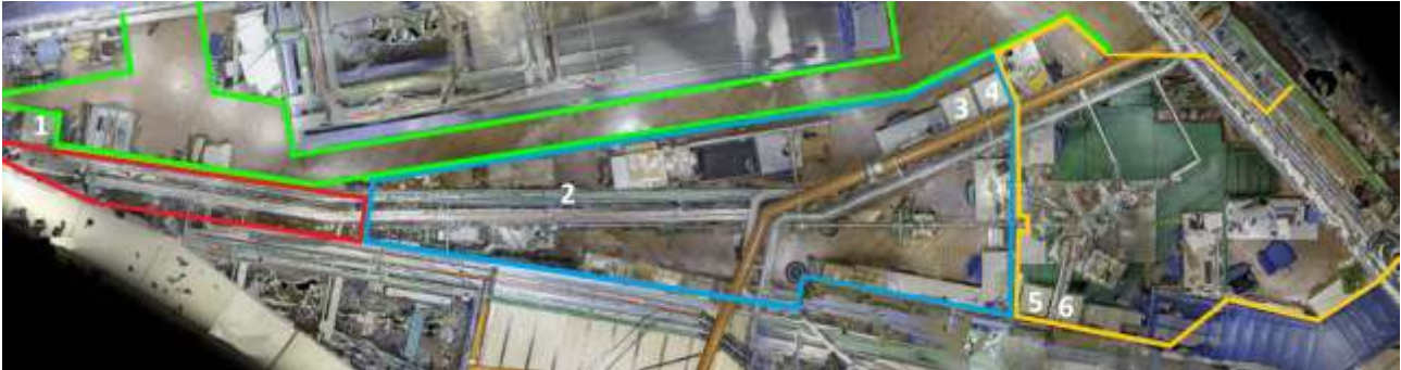
Figure 1: Top view of MSB. Front-end and first mirror hutch area (red), the rest of the beamline area (blue), end station area (orange), escape route (green). Numbers indicate 6 racks containing control electronics.
